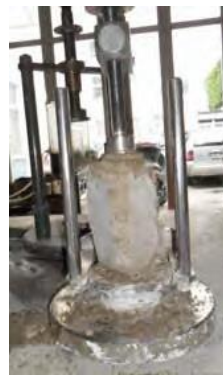
(h) specimen trimming
