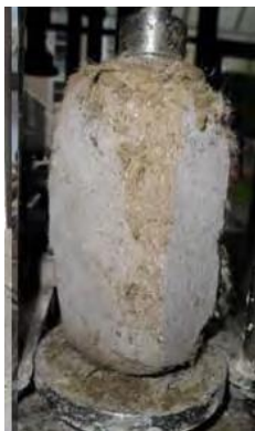
(g) specimen trimming
